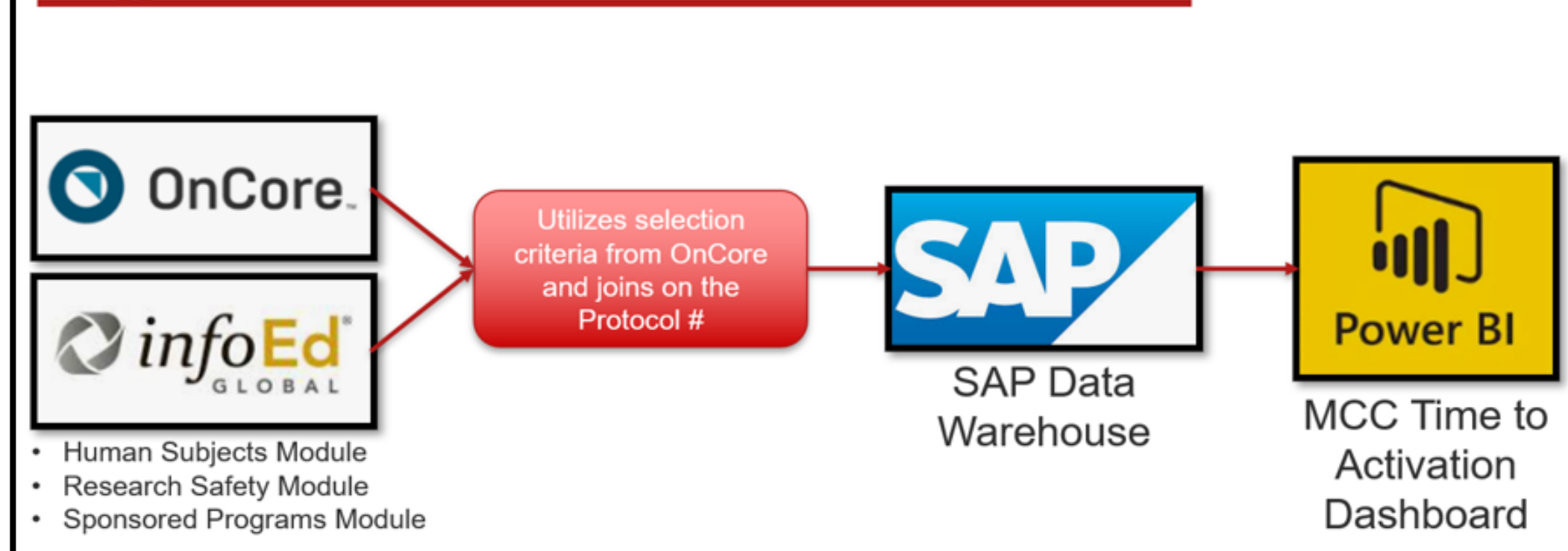
Figure 1. High Level Solution Architecture displays the IT solution that transforms transactional data from institutional systems into a dashboard hosted by PowerBI.
